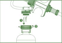
Holding syringe upside down, pierce septum with needle. Screw to tightly lock bottle.
