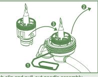
Push clip and pull-out needle assembly. Insert new needle assembly.
