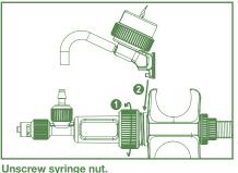
Unscrew syringe nut. Insert vial holder body until abutment.
