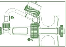
Tighten casing nut to lock vial holder body. Connect tubing to in take valve.
