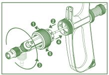
Place intake valve in vertical position.
